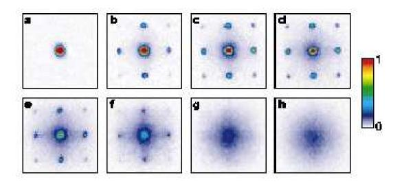
Absorption images (in 3D) of multiple matter wave interference patterns. (a)  $U = 0E_r$ , (b)  $U = 3E_r$ , (c)  $U = 7E_r$ , (d)  $U = 10E_r$ , (e)  $U = 13E_r$ , (f)  $U = 14E_r$ , (g)  $U = 16E_r$ , (h)  $U = 20E_r$  ( $E_r = \frac{\hbar^2 k^2}{2m}$ )
