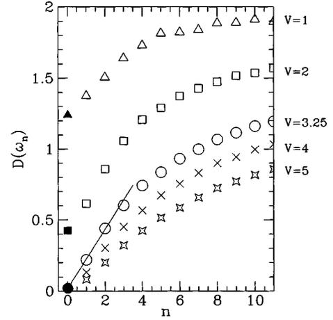
FIG. 2.  $D(\omega_n)$  as a function of  $n = \omega_n/2\pi T > 0$ , for fixed  $T = 0.1$  and various disorder strengths. The extrapolated value  $D(\omega_n \rightarrow 0)$  is shown as a solid symbol at  $n = 0$ . For small  $V$  this extrapolation yields a nonzero  $D$  indicating a SC. For the metallic system  $V = 3.25 (\approx V_c)$  we obtain  $\sigma_{dc}$  from the slope at small  $n$ ; see text.
