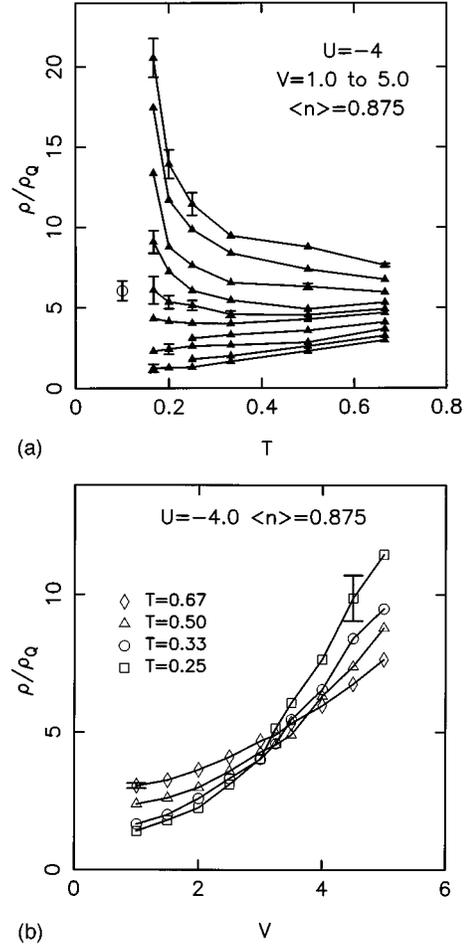
FIG. 3. (a) dc resistivity, obtained from Eq. (9), as a function of temperature, with disorder strength  $V = 1$  (lowest curve), 1.5, 2, 2.5, 3, 3.25, 3.5, 4, 4.5, and 5 (top curve). The point at  $T = 0.10$ , for  $V = 3.25 \approx V_c$ , is obtained from  $D(\omega_n)$ ; see Fig. 2. (b)  $\rho_{dc}$  as a function of disorder  $V$  for various temperatures  $T$ . Representative error bars are shown.
