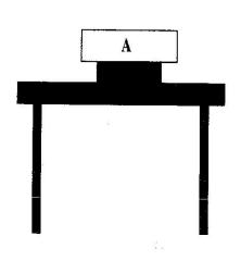
Fron A + WA = 0 FAORB = -17.64 N Fron A = WA = +1.8(9.8) = 17.64 N Frable on B + Wg + FAORB = 0 Frable on B = 5.88 + 17.64 = 23.52 N Fron lable = -23.52 N
