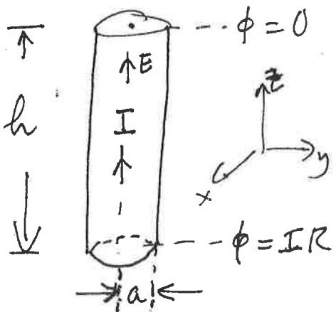
If the wire has resistance  $R$ , the potential drop is  $IR$  as shown and
