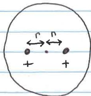
From Gauss' law, the electric field inside a sphere of constant charge density  $\rho$  is
