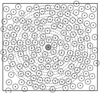
Count the number of particles centers found in each ring of size dr (here equal to b) and make a table:
